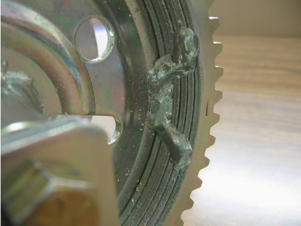
Welded gear laminates are stronger and more rigid than rivets.
