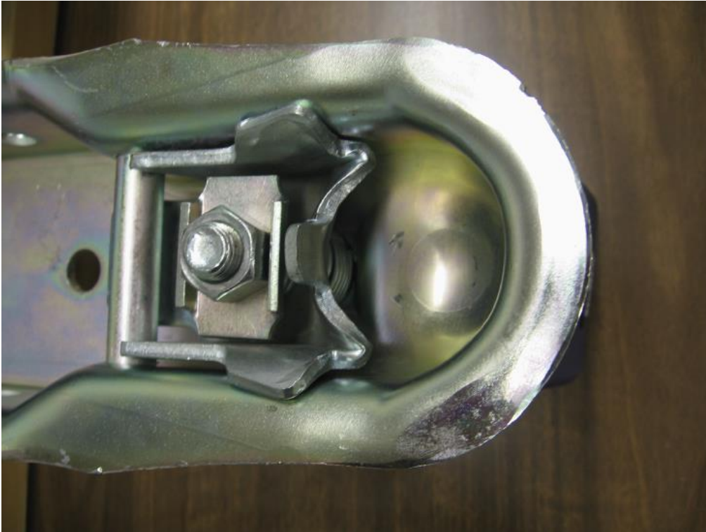
Patented ball clamp in DL couplers and fingertip adjustable nut.
