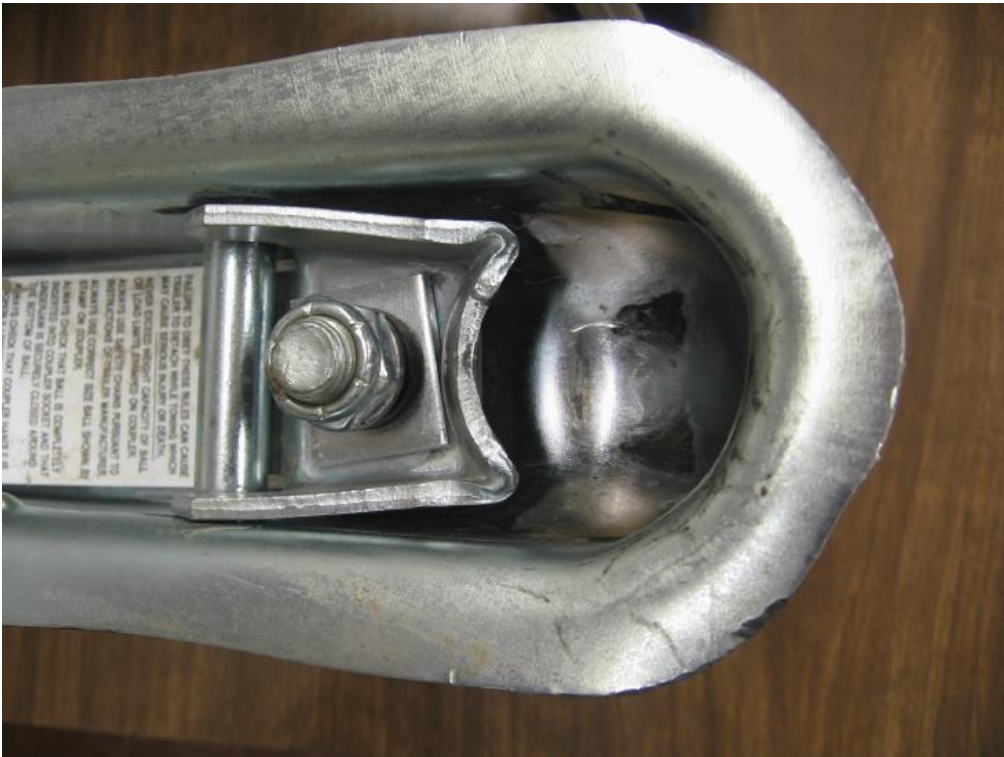
Smaller clamp in competitive couplers and locknut requiring tools.
