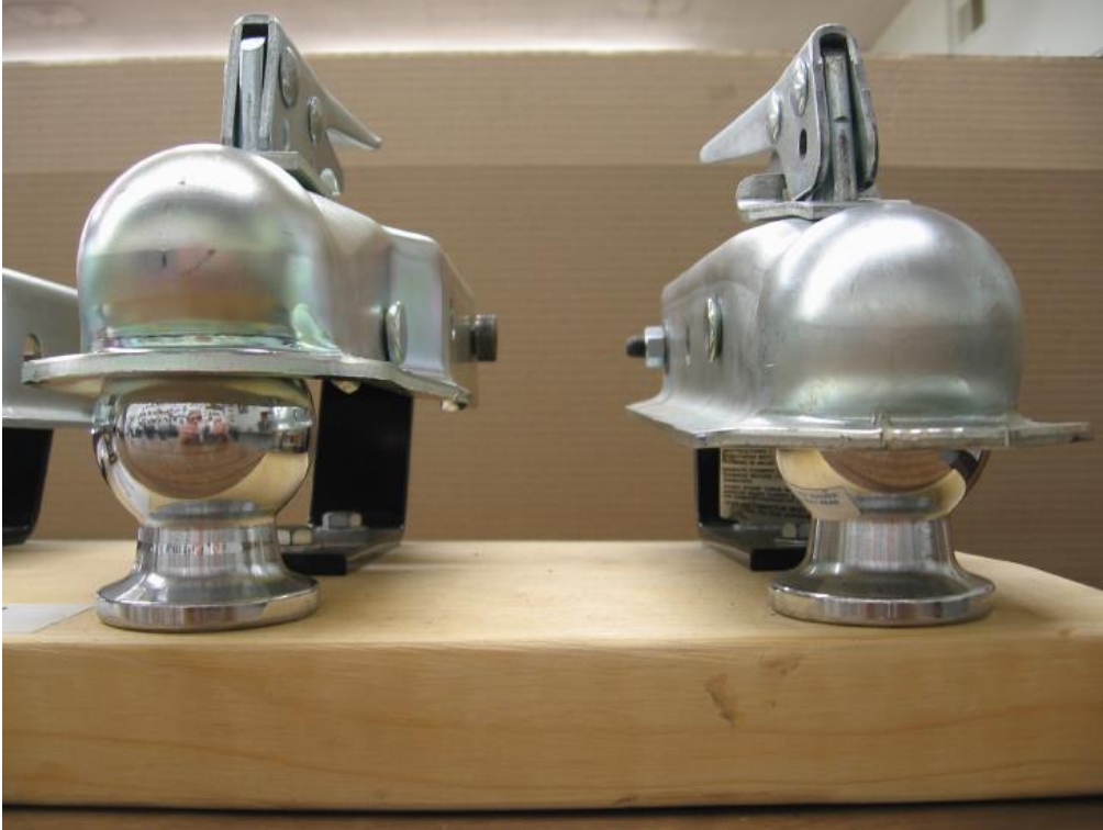
Left - Patented clamp in DL couplers prevents ball entry when miss-coupled. Right - Ball enters competitive coupler half way when miss-coupled. Easily towed.
