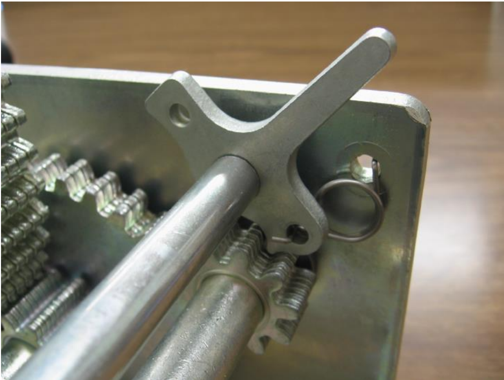
Reversible ratchet in larger winches is simple and less confusing to operate.
