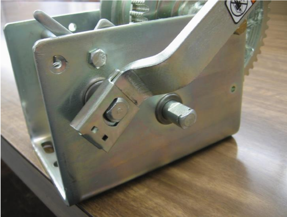
Two speed models use quick attach handle with spring loaded retaining clip.
